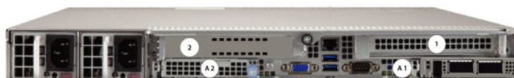
1. PCIe 4.0 x 16 slot full-height, half-length (CPU2); 2. RAID Card; A1. dual 100GbE/QSFP28; A2. PCIe 4.0 x 16 OCP 3.0 SIOM slot (CPU2)
