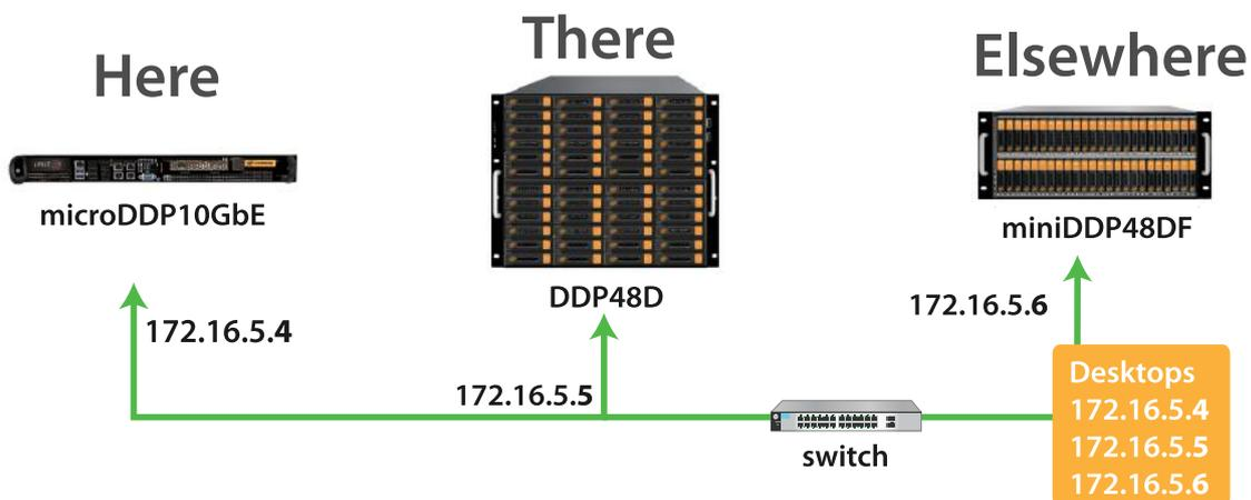
Individual DDP cluster nodes can be distributed over the network across separate physical and geographic locations while remaining within the DDP cluster. If necessary, a single DDP server can be removed from a cluster, used as a standalone device elsewhere, and...
